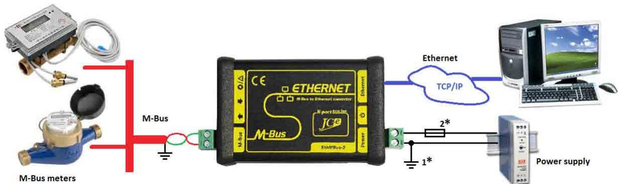
Typical wiring of the converter with M-Bus devices, power supply and Ethernet network connection.
