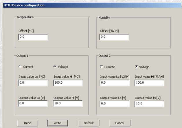
With clicking on the button "READ" the configuration values from the flash memory of sensor are read. With clicking on the button "CANCEL" the configuration window gets closed.
