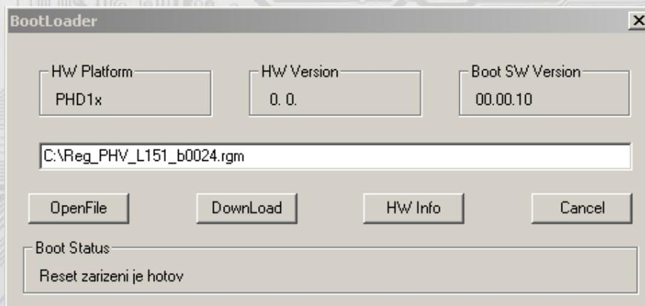
The work with application is conditioned by insertion of the jumper J6 (authorisation for configuration values recording). Using the button "OpenFile" the new application FW is chosen and using the button "DownLoad" the FW variation gets started, being automatically controlled by PC and the device.
