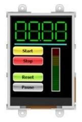
For the needs of the AMRobot platform it is possibile to use any display available, however it is recommended to use an intelligent graphic display by *4D Systems* that can be quickly configured by external master microcontroller (*Arduino* for instance) through serial interface (UART). It can also work as a standalone device. The choice of work mode is accomplished by a public configuration file available on *4D Systems* website.
