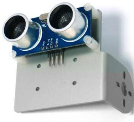
Optional version of pan/tilt head (for Raspberry Pi camera and ultrasonic distance sensor) - can be mounted together or separately on the head
