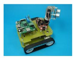
Particular robot versions differ in chassis configuration (2-wheel version, 4-wheel version and tracked drive system. Each configuration can be assembled on the same mounting board which is equipped with special spots and mounting holes to fasten the chosen motors and wheels. The user can choose two types of motors and different wheels. These are assembled on the same bottom mounting board.
