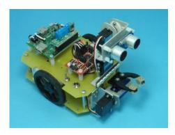
AMEX Mini Robot is a new, unique educational platform for building a mobile mini robot. The platform is designed in a way that provides a variety of configurations of mechanical and electronic part of the robot.
