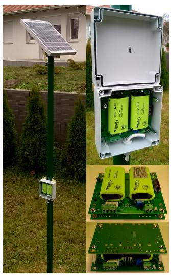
V1 variant: - Add-on board with sandwich structure, connect high row pins - IP67 protection Fibox Euronord housing, sandwich structure
