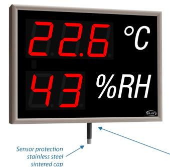
The **NDA 100/3-2 THS R L20 230AC USB** is an electronic monitoring device which measures and displays air temperature and humidity on a large format.
