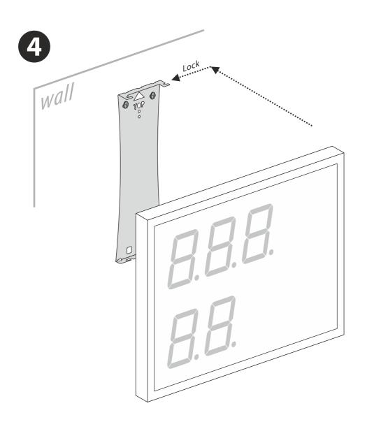
Insert display onto the mounting bracket and latch it in by moving it to the left side.
