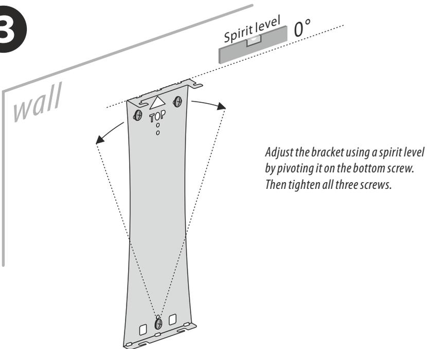
*Adjust the bracket using a spirit level by pivoting it on the bottom screw. Then tighten all three screws.*
