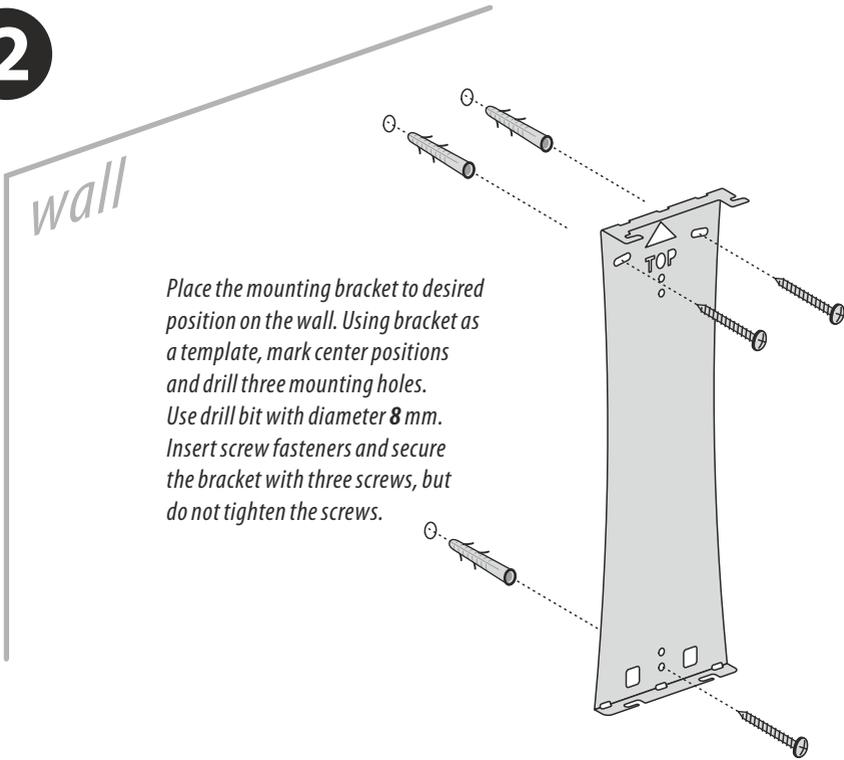
*Place the mounting bracket to desired position on the wall. Using bracket as a template, mark center positions and drill three mounting holes. Use drill bit with diameter 8 mm. Insert screw fasteners and secure the bracket with three screws, but do not tighten the screws.*
