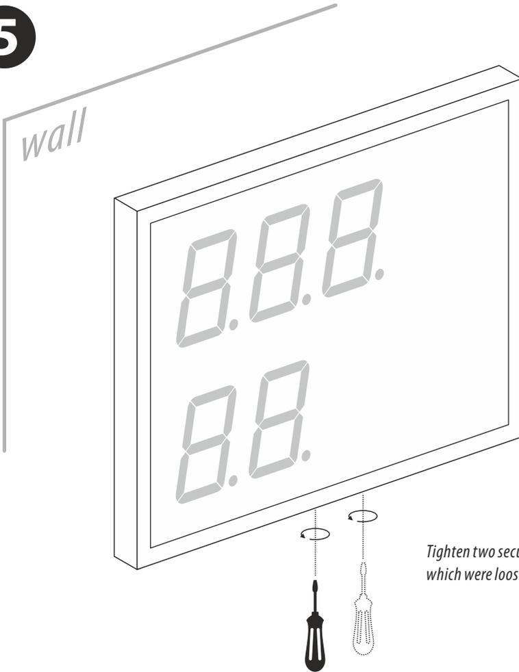
*Tighten two securing screws,
