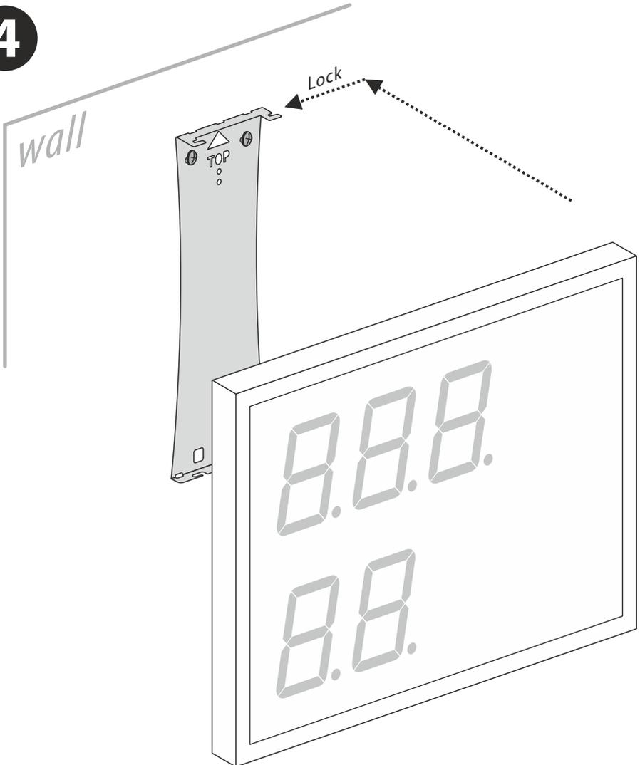
*Insert display onto the mounting bracket
