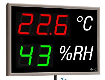
The **NDA 100/3-2 THS RG L20 PoE LAN** is an electronic monitoring device which measures and displays air temperature and humidity on a large format.
