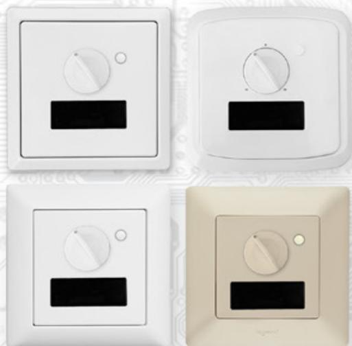
The E-33 indoor device is equipped with a wireless temperature sensor communicating according to the EnOcean radio standard. It allows setting the correction of the desired temperature using a rotary knob and is also equipped with a presence button.
